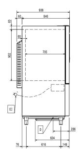
Drain ΕI Electrical inlet (power)
